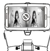
The central line of the phone doesn't line up with the marked line on the lid
